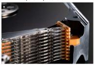
Suspensions for HDDs are unique spring products, holding the read-write head in HDD devices.
