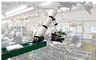
Position correction with 3D cameras + Automatic supply to conveyor lines by collaborative robots
