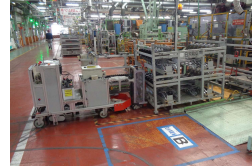
Automation of transport using automated guided vehicles (AGVs)/autonomous mobile robots (AMRs)
