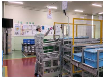
Using a mechanism cart, items are moved onto the cart by their own weight, falling onto the cart
